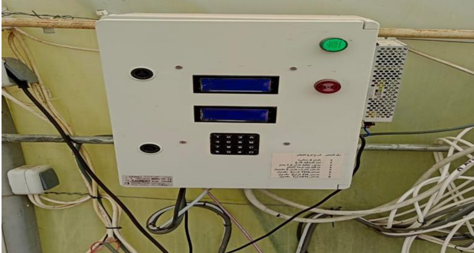
Control units and pump system to add the Plant nutrition solution (A, B, and C).
